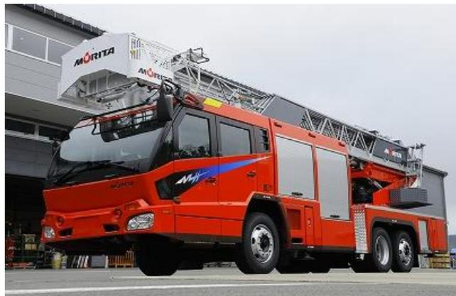
These Super Gyro Ladder MLL Series trucks with top articulated ladder and water piping offer dramatically improved ladder retraction/extension speed and significantly expanded work range along with reduced ladder weight. The ladder trucks, designed with a great emphasis on the ease of use, are also equipped with a new control system that offers the fastest and the most efficient rescue and firefighting possible.
