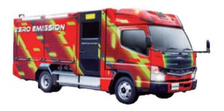
Japan's first\* electric fire fighting vehicle with zero emissions, low noise and low vibration. The independently developed ePTO (pump drive system) and e-Fire Pump (dedicated EV pump) achieve high energy efficiency.
