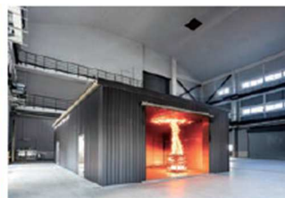
● Simulated Apartment Reproduction and verification of actual firefighting environments
