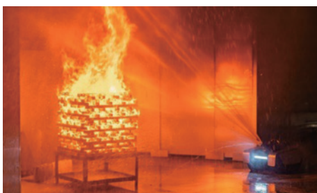
Combustion and extinguishing experiments (Simulated Apartment)
