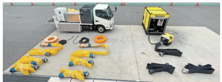
Dewatering pump useful for dewatering at sites of inundation and submergence
