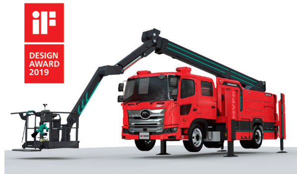
Multi-Purpose Firefighting Vehicle with a 21m Aerial Platform, MVF21
