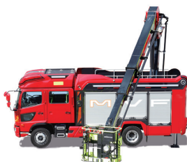
Multi-purpose fire fighting vehicle with 13m aerial platform
