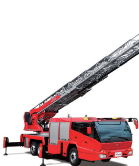
Ladder truck with 30m top articulated boom
