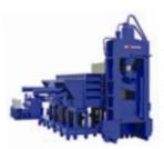
MORITA ENVIRONMENTAL TECH CORPORATION developed a new cutting machine for large-sized scraps and started selling it in fiscal 2008. By incorporating oil pressure system, the cutting speed capacity was dramatically improved to four times a minute (no load). Development with a focus on the
