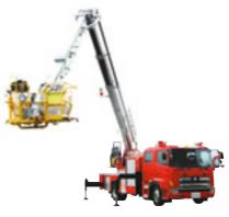
Further, the telescopic/refractive boom capable of lowering itself below the ground level helps better avoid electric poles and other high-altitude obstacles that can often hinder rescue operations, as well as lifesaving operations at river and sea. Morita will continue to present technologies that are useful and effective in rescue operations.
