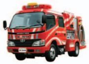
with compressed air causes it to foam. This equipment maximises the surface area of the water which enables fire-fighting with only small amounts of water. The current Miracle CAFS Car carries 600 liters of water and 2 liters of fire-extinguishing agent which provides a fire-fighting capacity equivalent to some 10 tons of water.
