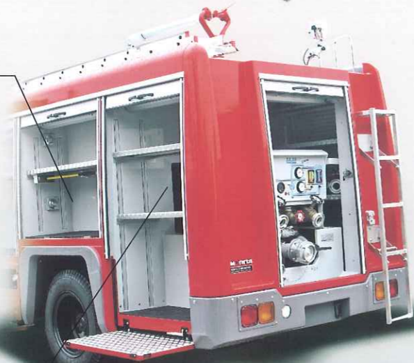
OTHER PUMPS Large Volume Pump Pump model: MD260A Performance: 4,200L/min at total head 8 bar
