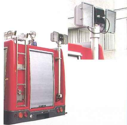
Extendable Lighting Tower Halogen 1000W×2pcs 6M high from the ground
