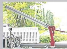
FOAM TURRET NOZZLE 1000L/min at 7bar
