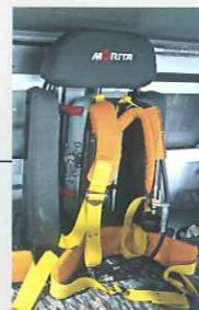
SCBA Seat (Self Contained Breathing Apparatus) SCBA Seat is installed on the backrests of the seats.
