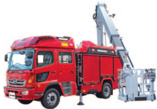
MVF Multi-Purpose Fire Fighting Vehicle with 13m Aerial Platform
