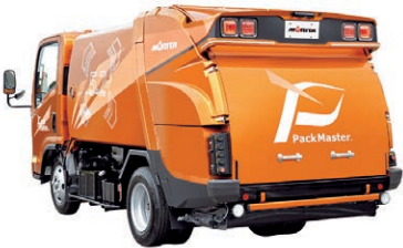
Pack Master rotary extrusion garbage collector
