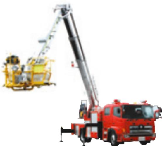
Further, the telescopic/refractive boom capable of lowering itself below the ground level helps better avoid electric poles and other high-altitude obstacles that can often hinder rescue operations, as well as lifesaving operations at river and sea. Morita will continue to present technologies that are useful and effective in rescue operations.
