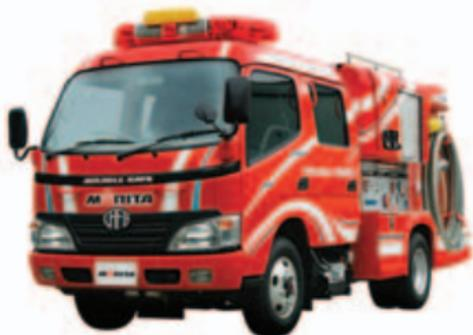
with compressed air causes it to foam. This equipment maximises the surface area of the water which enables fire-fighting with only small amounts of water. The current Miracle CAFS Car carries 600 liters of water and 2 liters of fire-extinguishing agent which provides a fire-fighting capacity equivalent to some 10 tons of water.
